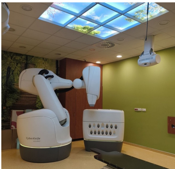
Figure 2. CyberKnife at the National Institute of Oncology, showcasing robotic non-coplanar beam delivery for stereotactic radiotherapy.
